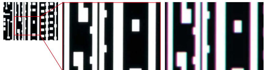
Apochromat optics (captured with SMZ1270+Plan Apo 1x/WF)
